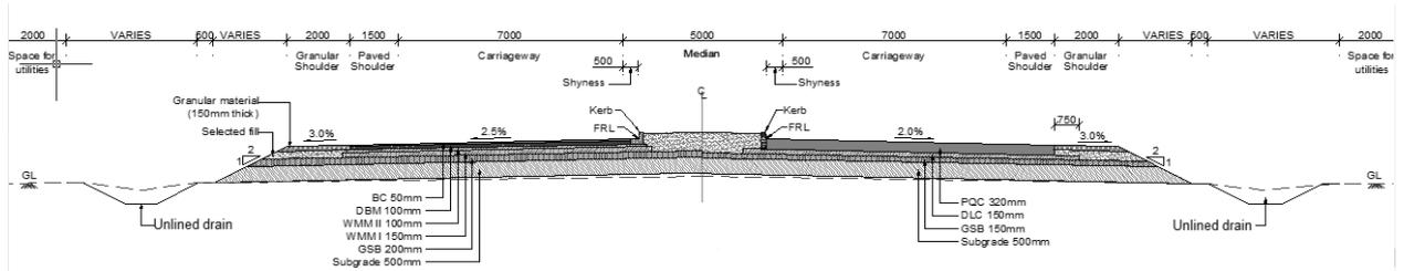
**Figure 2.15: TCS 1C.4- New Alignment / Realignment**
