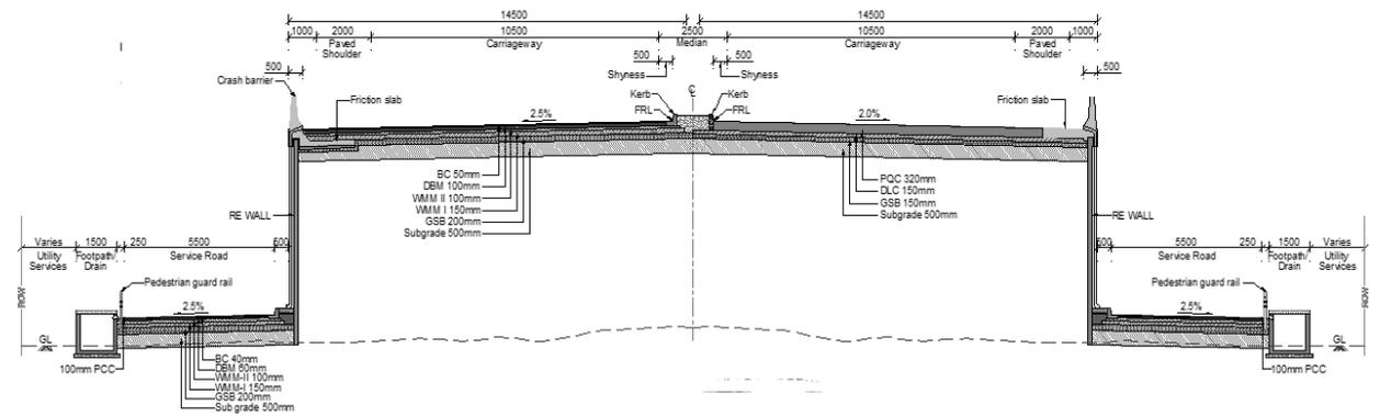
**Figure 2.21: TCS 8.4- Vehicular / Light Vehicular Underpass**
