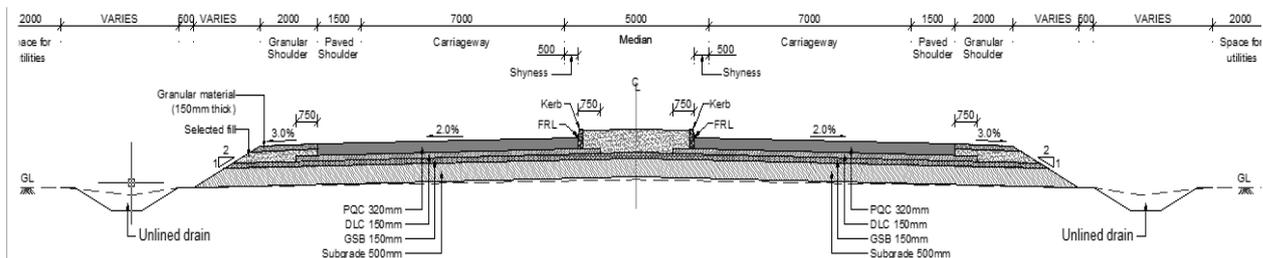
**Figure 2.13: TCS 1C.2- New Alignment / Realignment For 4 - Lane In Rural Area**
